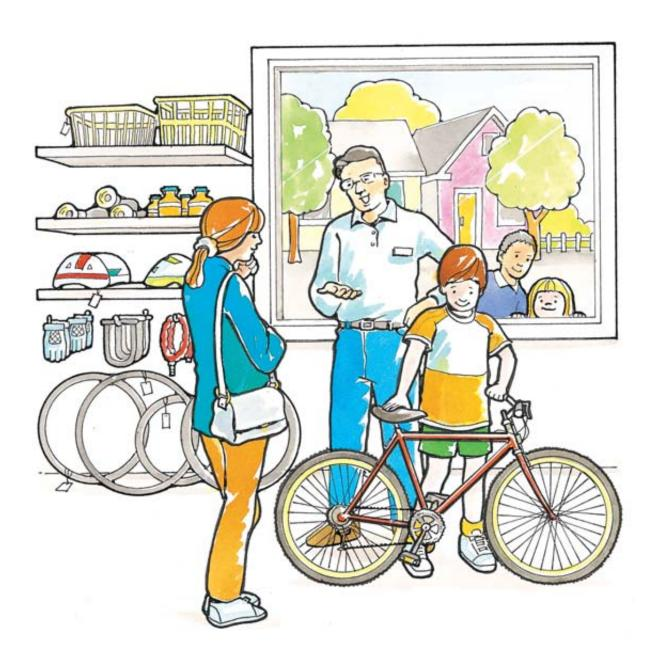
With both feet on the ground, you should be able to straddle the crossbar of the bicycle like this, with 2 to 5 cm (one to two inches) of clearance.
